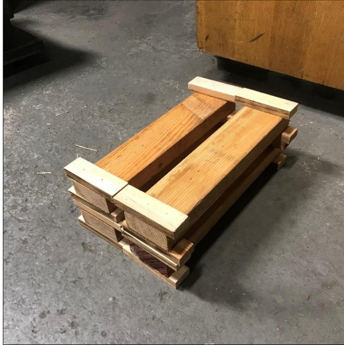
Typical Test Fuel Load Configuration
