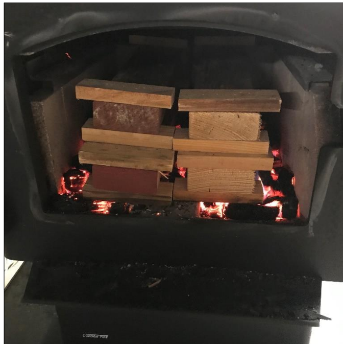
Typical Test Fuel Loaded in Test Stove
